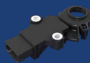
Sensor to measure the angular position of the brake, clutch or gas pedal.
