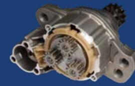
Internal geared plastic wheel for start/stop automation to reduce fuel consumption and CO<sub>2</sub>.
