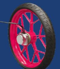
Wheel hub gears provide drive in electrically powered micro-vehicles in E-axes.
